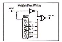
The realizable accuracy will be determined by how the logic is implemented and the associated propagation delays through it compared to the chosen delay time. Ideally, the external propagation delays should be small compared to the delay time, in which case the output pulse width will be close to the delay time used.
